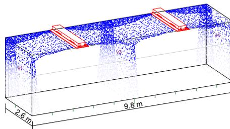
Figure 8. Chilled beam selections for meeting room in advanced case. Velocity V1 near the wall has reduced from 0,35 m/s (Fig 7.) to 0,25 m/s as well as the velocity between the chilled beam rows.
