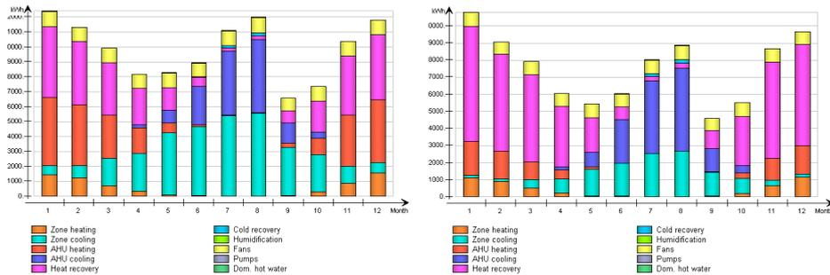
Figure 9. Monthly energy consumption breakdown in reference case (left) and in advanced case (right).
