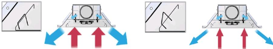
*Figure 1. Velocity control is located into a supply air slot of an active chilled beam, where it adjusts both the induction rate of a chilled beam and a slot opening. This guarantees a good throw pattern also with reduced amount of induced air.*
