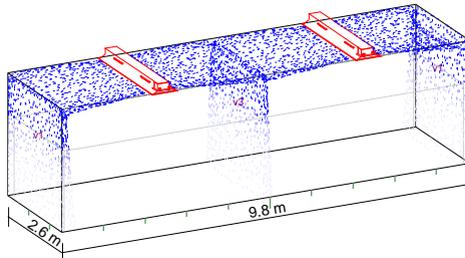
Figure 6. Chilled beam selection for reference office case. Velocity V1 presents the room air velocity near wall in an office space and velocity V3 presents the velocity in landscape office between the beams.
