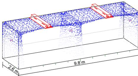
Figure 7. Chilled beam selection for meeting room in reference case.
