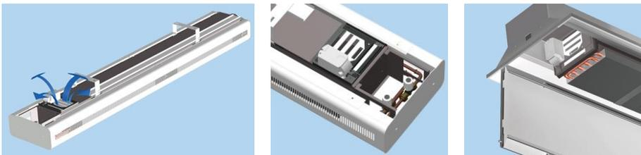
*Figure 2. Air quality Control unit is integrated into chilled beam to adjust the required extra air flow rate of a chilled beam. Minimum airflow requirement is supplied through nozzles. In case of a high maximum airflow rate, Air Quality Control unit on the top or inside of a chilled beam can be motorized (e.g. meeting rooms).*
