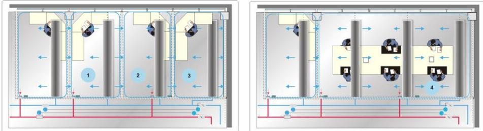
Figure 3. Typical floor layout where both Velocity Control and Air Quality Control are used to adjust the operation of each chilled beam to provide right air volume and throw pattern both as an office room (beams 1, 2, and 3), open-plan office (beams 1, 2, and 3), and as a meeting room (beam 4).
