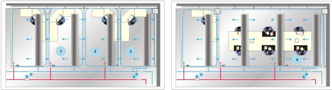
Figure 5. Typical floor layout where both velocity control and air quality control are used to adjust the operation of each chilled beam to provide right air volume and throw pattern.
