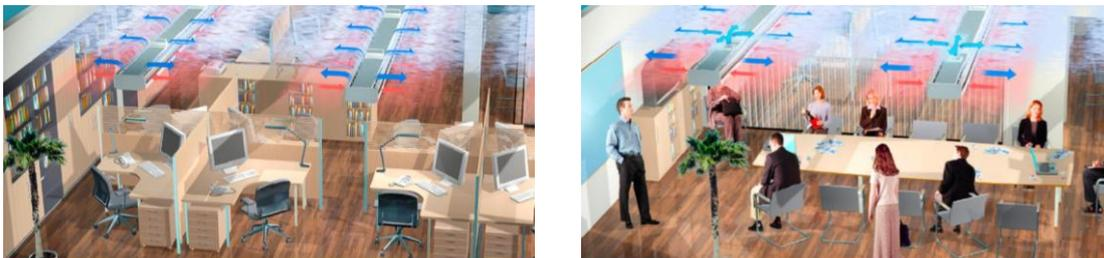
Figure 4. Air quality (HAQ) control unit to adjust the required extra air flow rate of a chilled beam. Minimum requirement is supplied through nozzles (left). In case of a high maximum airflow rate, this HAQ unit on the top of a chilled beam can be motorized (e.g. meeting rooms).
