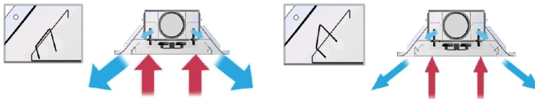
Figure 3. Velocity control is located into a supply air slot of an active chilled beam, where it adjusts both the induction rate of a chilled beam and a slot opening. This guarantees a good throw pattern also with reduced amount of induced air.
