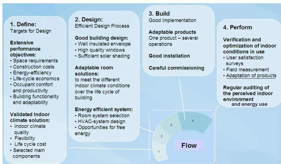
Figure 1. Total lifetime management process of indoor climate quality was developed. There is more focus in target setting and a new business model of verifying indoor conditions was introduced.
